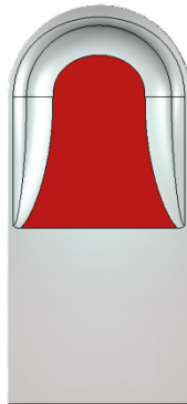
FIG. 4. Orthotics insole area subjected to filling modification with different structures and degrees of filling
