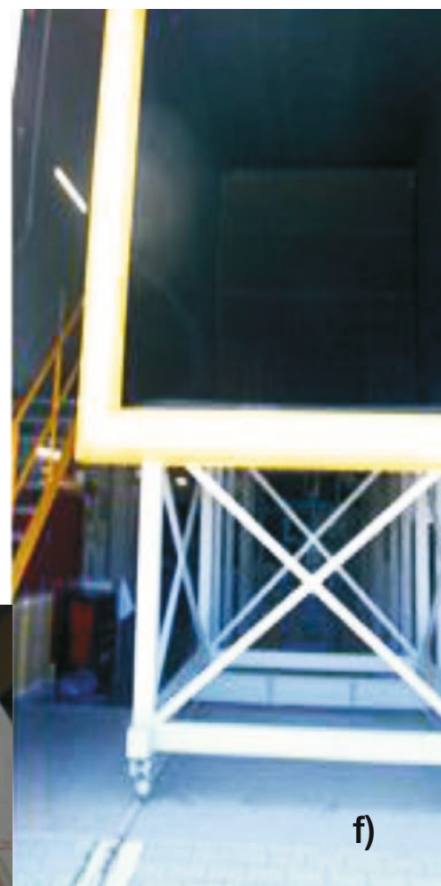
Fig. 5a-g. PAS Research Centre, Energy Conversion and Renewable Resources KEZO, Jablonna near Warsaw, Poland a) buildings B2,B2/1 and Laboratory of Wind Energy L3, b-g) is provided an open flow low speed wind tunnel designed to testing small scaled wind turbine (equipped with an open low-speed wind tunnel that is equipped with two independent measurement chambers; required for testing small wind turbines or models). KEZO can also realize numerical simulations supporting analysis and design of wind turbine and investigations of other wind energy related issues; source: photo by the author 2019
