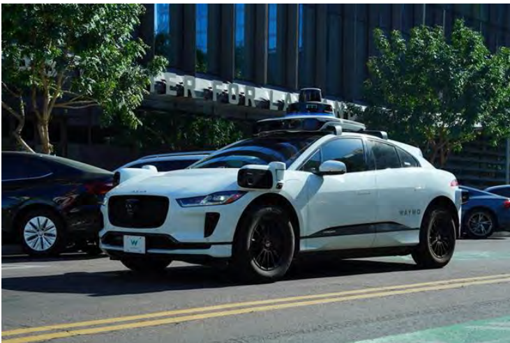
Fig. 2. Autonomous robotaxi by Waymo Via, Jaguar I-PACE model
