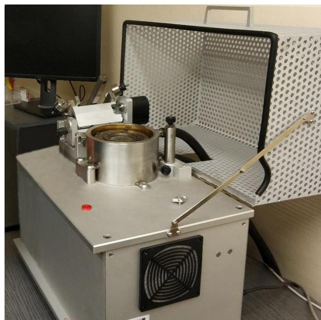
Fig. 1. High temperature Anton Paar tribometer TRB<sup>3</sup>
