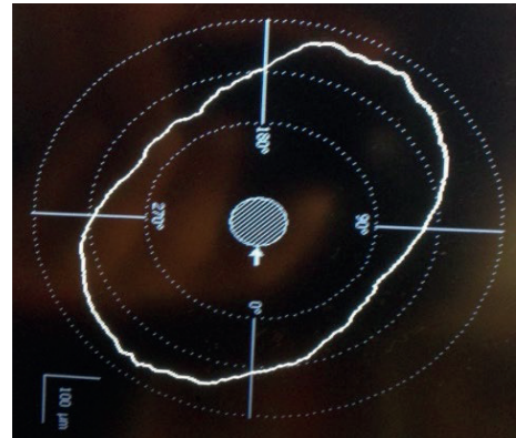
Fig. 6. Housing top-sealing face profile
