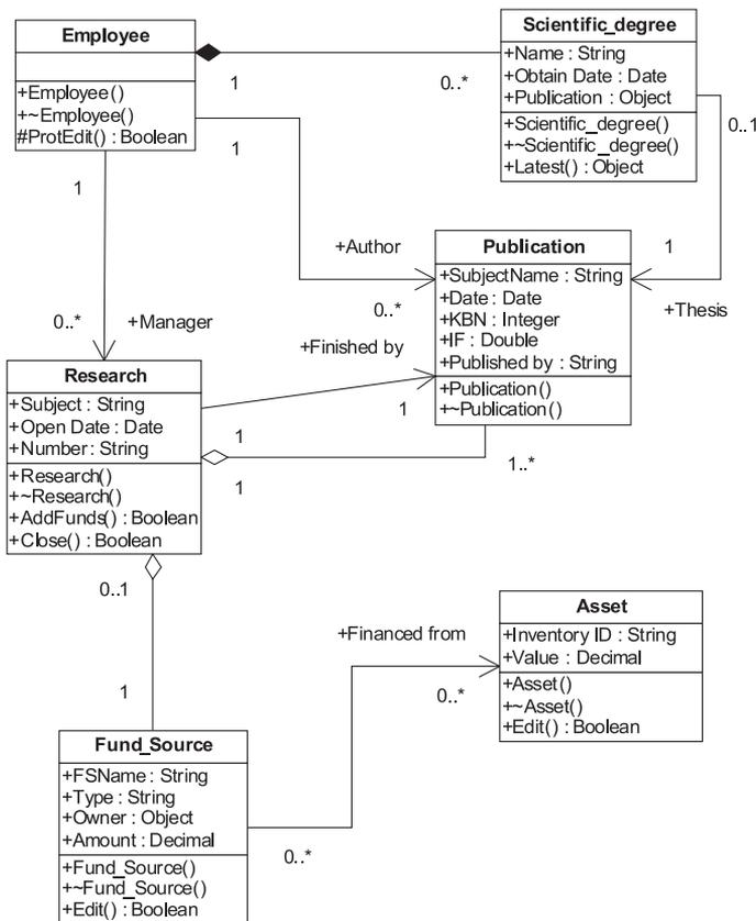
Fig. 7. Class diagram of scientific data
