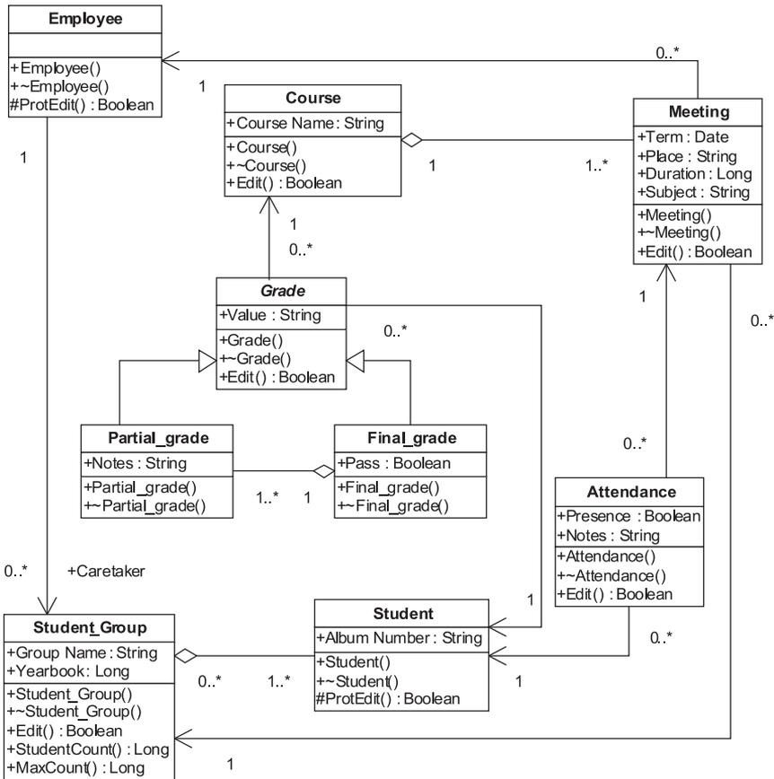
Fig. 5. Class diagram of student evaluation data
