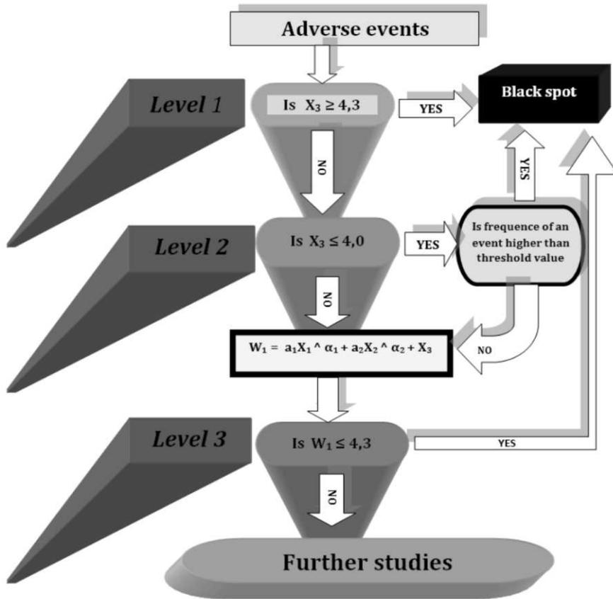
Fig. 3. Model of proceeding when determining black spots
