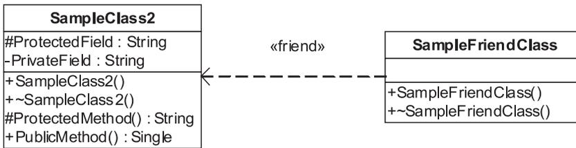
Fig. 2. Simple class diagram with friend and different function/members kinds
