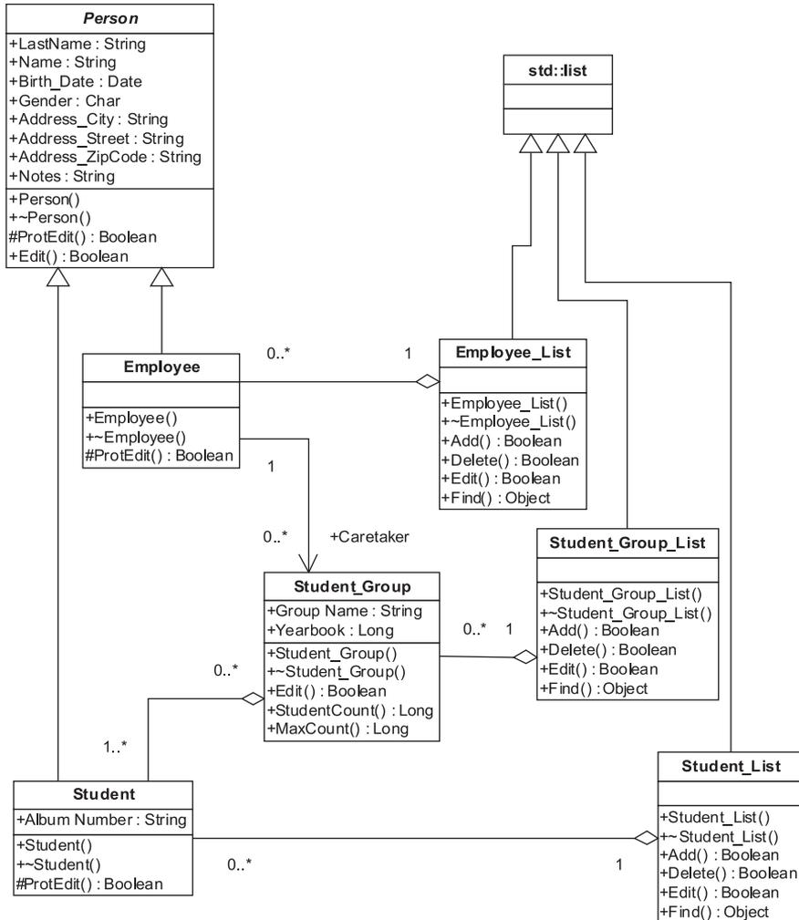
Fig. 4. Class diagram of list containers
