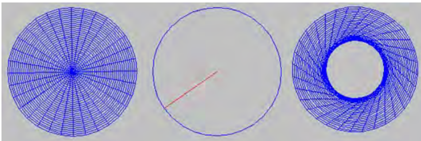
Figure 3.2: Three surfaces resulting from the rotation of the straight line around a given straight line (top view), prep. E. Koźniewski
