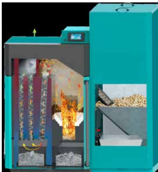
Fig. 6.13. Pellet boiler (Source: WEB-6)
