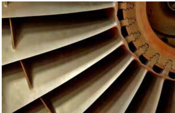
Fig. 7.10. The Impeller's blades of the turbine's lower pressure part (Source: WEB-6)
