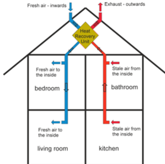
Fig. 8.20. An example of using HRV in a single-family home (Source: own elaboration)
