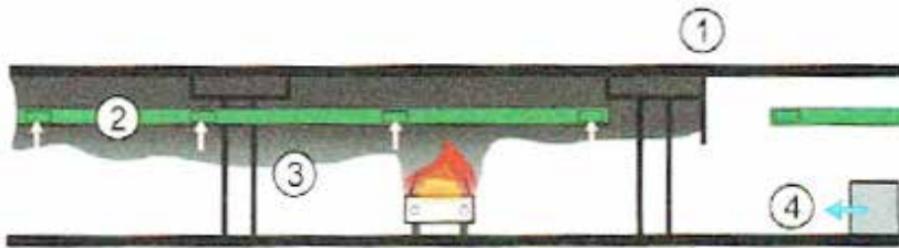
Fig. 9.6. Principles of operation of the smoke ventilation duct system (Source: based on data from Węgrzyński & Krajewski, 2015)
