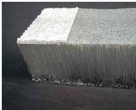
Fig. 3.17. Transparent insulation designed for connecting with the ETICS system (Source: Kisielewicz, 2010)
