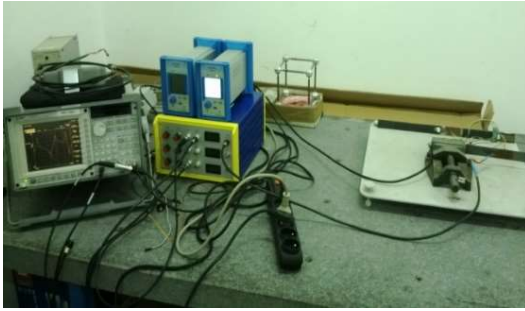
Fig. 4.2. The photo of test rig during identification procedure (left), the frequency response function of the smart beam in the selected frequency range 10-410 Hz (right)
