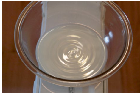
FIG. 6.7B. Standing waves formed on the surface of milk contained in a glass bowl ( https://cnx.org/contents/TqqPA4io@5.93:_jcAMgg6@5/16-6-Fale-stoj%C4%85ce-i-rezonans )
