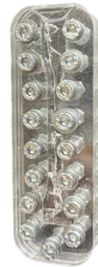
Fig. 3. Shells for shell-cast specimens
