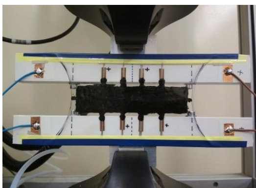
Fig. 4. Mounted DEG sample on the test rig
