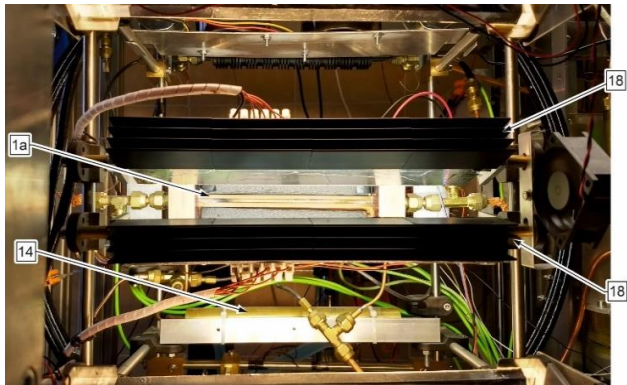
Fig. 3. View of the measuring module with mini-channels, markings: 1a – mini-channel, 18 – radiator of the LED illuminator, other markings as in Fig. 1.
