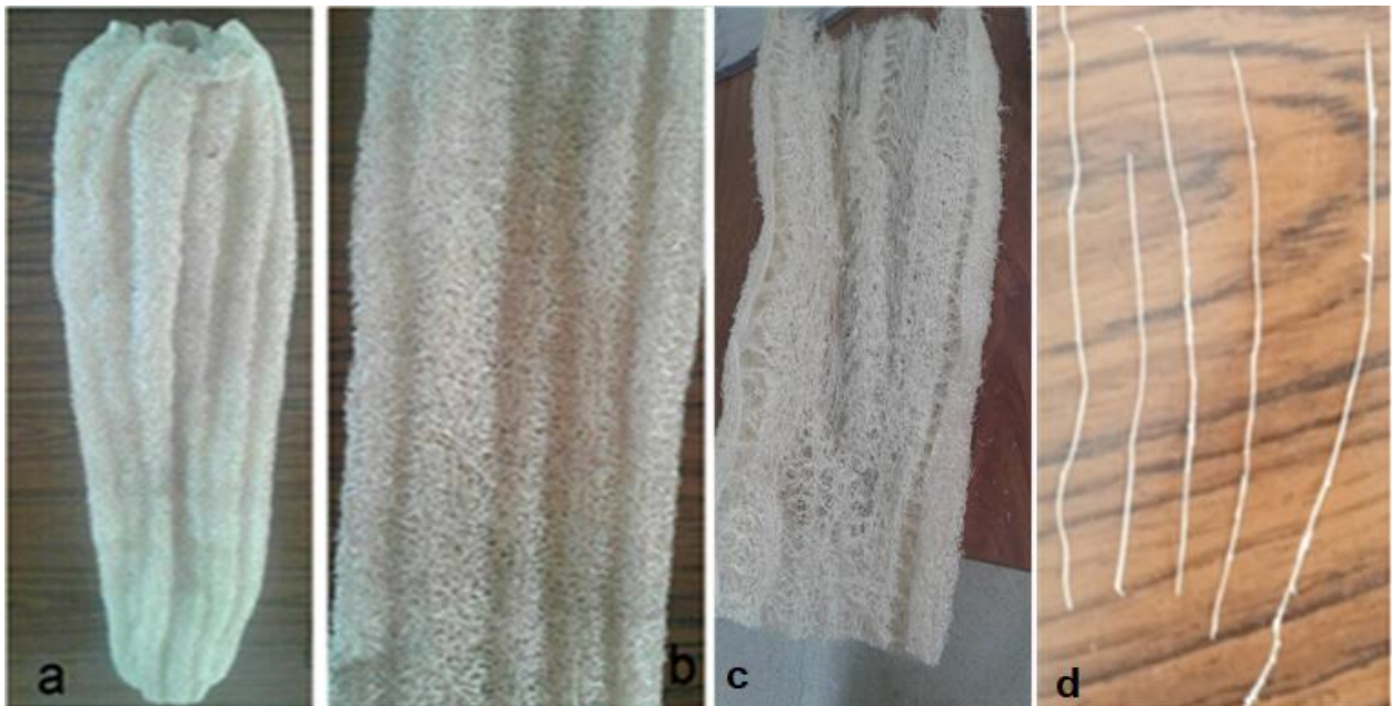
Fig. 2. (a) Luffa sponge, (b) The portion of the luffa open as mat, (c) luffa mat and (d) luffa fibres
