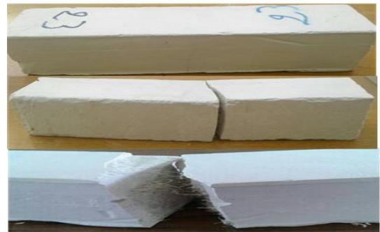
Fig. 14. Failure stages of plaster reinforced with mats of long unidirectional Luffa sponge fibers
