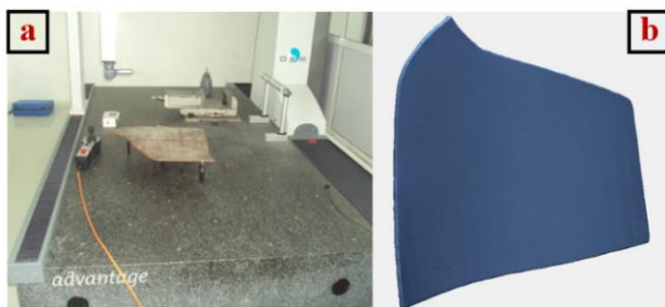
Fig. 1. (a) Impeller Blade; (b) Cloud data from (CMM) coordinate measuring machine
