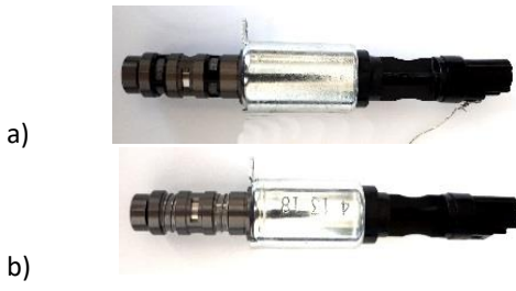
Fig. 7. A comparison of hydraulic solenoid valves. Ford's design (a) and a prototype solenoid valve design (b)
