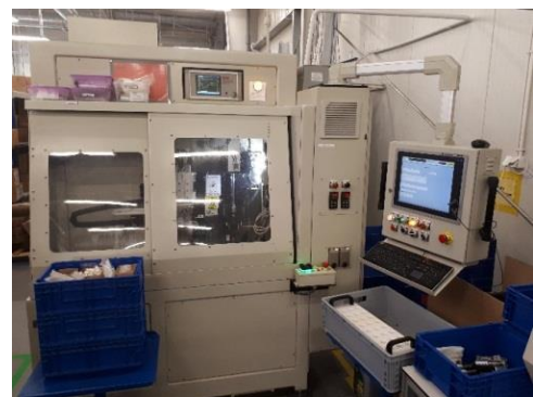
Fig. 4. Test stand for testing hydraulic solenoid valves
