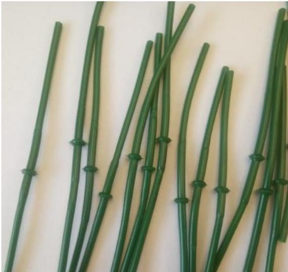
Fig. 7. Belt samples with flashes, prepared for the study
