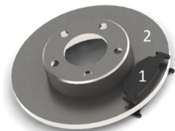
Fig. 1. Disc brake friction pair: 1 – brakepads 2 – corresponding brake disc
