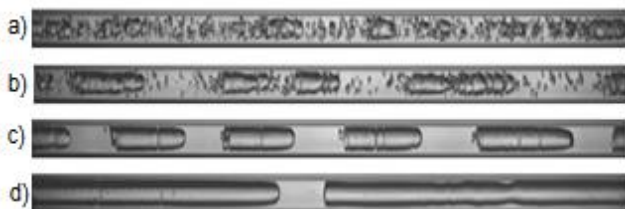
Fig. 3. Photos of the selected flow cases with increasing water volume flow rate q [l/min]: 0.216 (a), 0.145 (b), 0.071 (c), and 0.012 (d), respectively. The air volume flow rate was fixed to q_a = 0.1 l/min.
