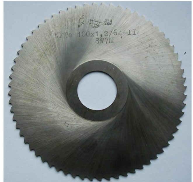
Fig. 6. NFTe 100x1.2/64-II circular slitting saw
