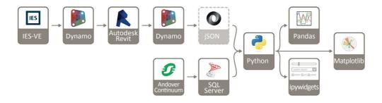
Fig. 6. Building energy calculation path in the BIM environment Source: (Gerrish et al., 2017).
