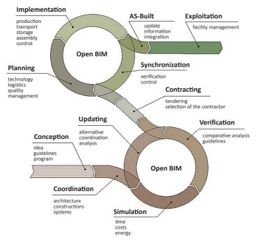
Fig. 2. Building process using the BIM method
