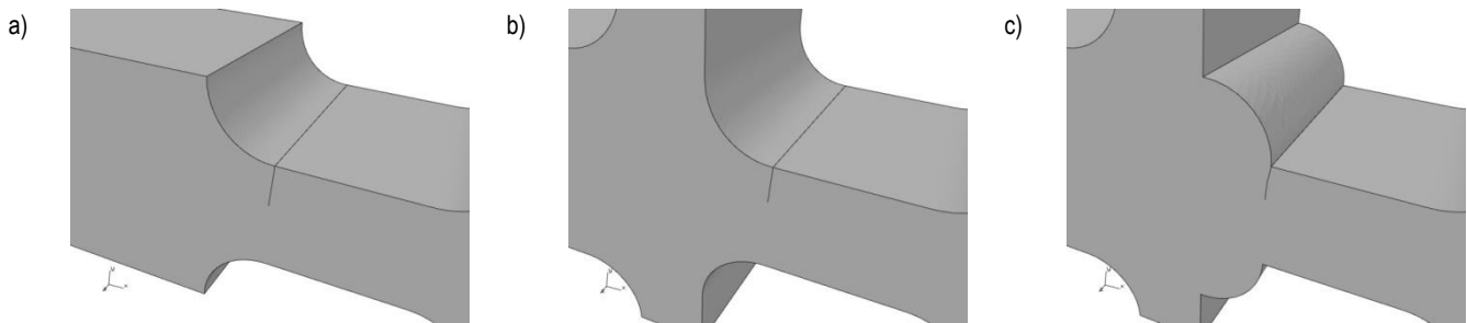
Fig. 5. Specimens with numerical calculation cracks: a) solid, b) with concave welds, and c) with convex welds
