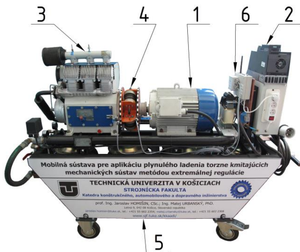
Fig. 2. The newly built mobile device for extremal control presentation: 1 – electromotor MEZ 4AP132M-4, 2 – frequency converter Sinamics G120C, 3 – piston compressor ORLIK 3JSK-75, 4 – pneumatic tuner 4-2/70-T-C, 5 – mobile platform, 6 – electronic extremal control system
