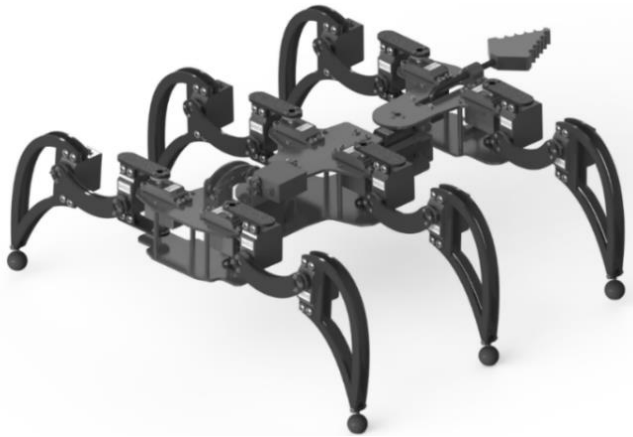
Fig. 2. 3D model of the hexa-quad bimorph walking robot in HEXAPOD configuration
