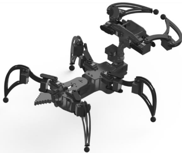
Fig. 3. 3D model of the hexa-quad bimorph walking robot in QUADRUPED configuration
