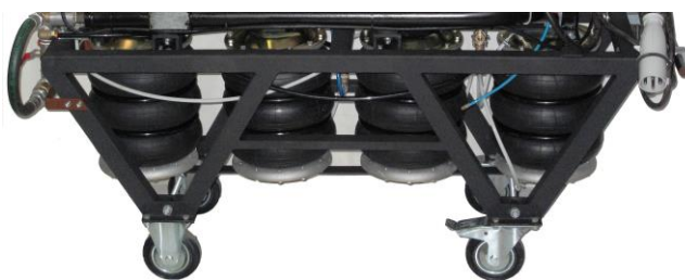
Fig. 3. The mobile platform with 4 air springs Rubena 340/3
