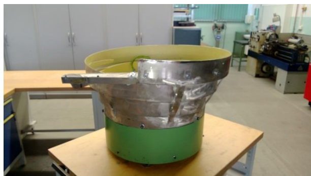
Fig. 1 Bowl feeder for testing
