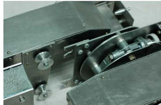
**Fig. 11.** Docking mechanism
