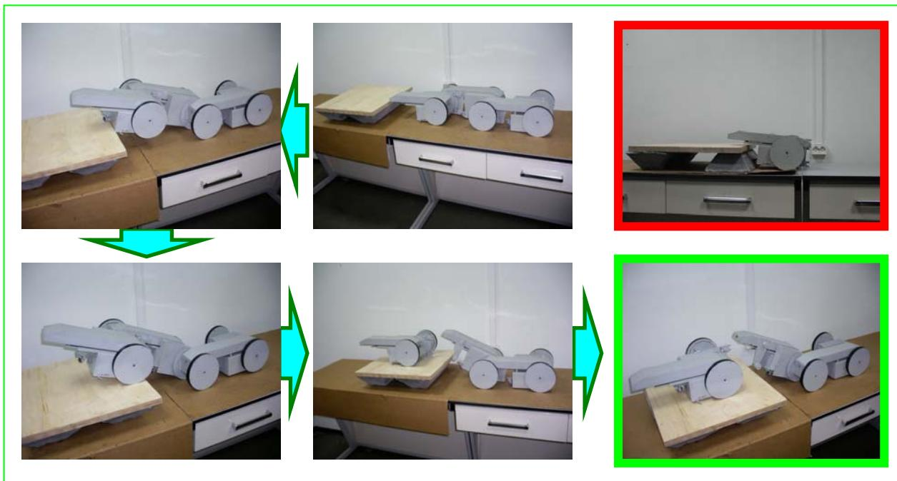
**Fig. 14.** Overpassing of a ledge
