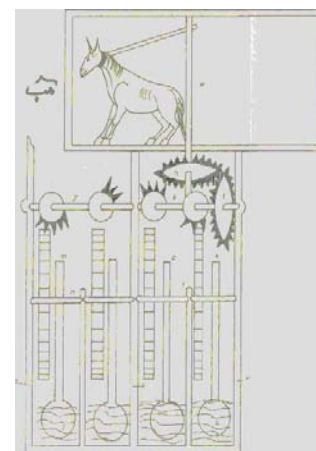
Fig. 4. 4 Effective water rising system (4 stroke cylinder)
