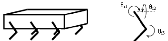
Fig. 1. The hexapod mobile robot (a); The variables of the leg i (b)
