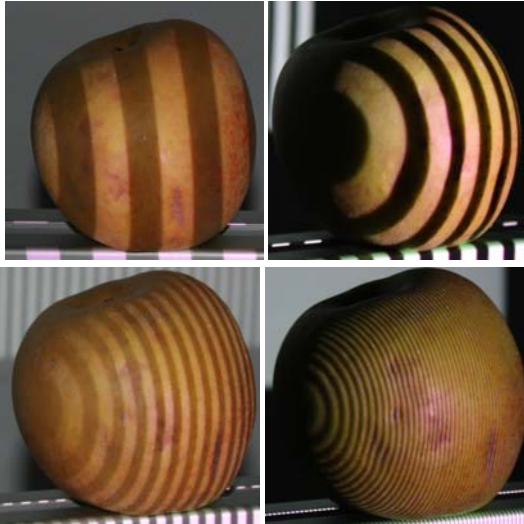
Fig. 7. Exemplary images of four Gray coded sine patterns with phase FN2\pi calculated from them
