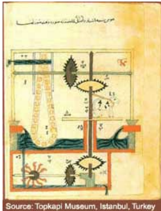
Fig. 1. Mechanical pump by Jazari
