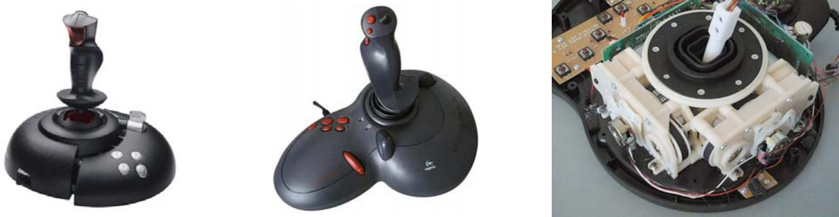
Fig. 4. Examples of low-cost haptic devices: the Microsoft SideWinder and Logitech Wingman force-feedback joysticks (from the left) and the internal view on electric actuators
