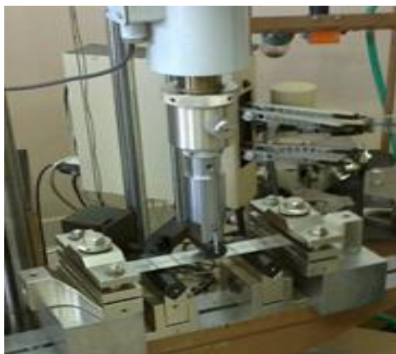
Fig. 5. The bending fixture on the testing machine TIRAtest 2300
