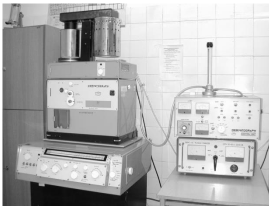
Fig. 4. View of the Paulik-Paulik-Erdey type apparatus (derivatograph) for thermogravimetric tests
