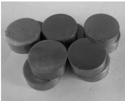
Fig. 2. Examples of samples prepared for ball-cratering tests
