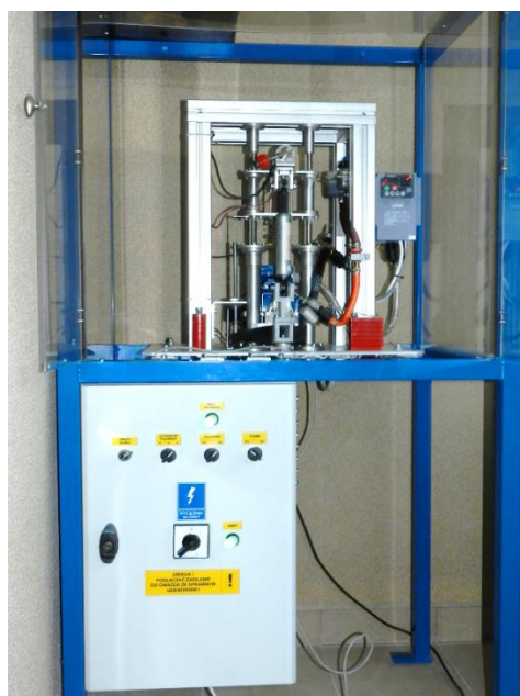
Fig. 2. Real view of EHDVA system with SMA oscillator's spring
