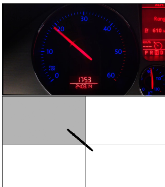
Fig. 1. Example of RPM pointer detection steps. Original video frame image, segmented pointer and divided dial with selected quarter highlighted.
