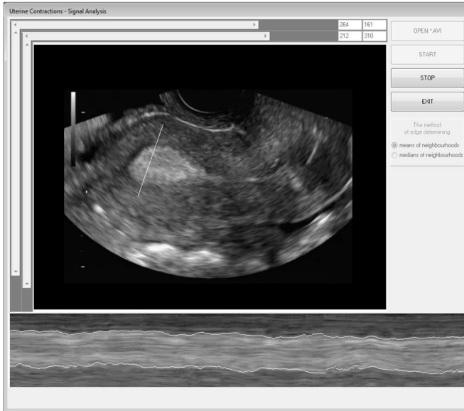
Fig. 1. Upper section of the figure – optimal setting of the gate on the uterine sagittal cross section. Lower section – image resulting from automatic detection of endometrial interface (marked by bright lines)
