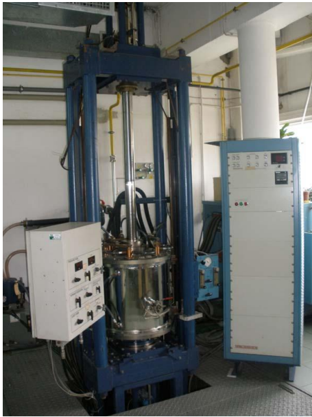
Fig. 1. Thermal Technology Astro uniaxial hot press
