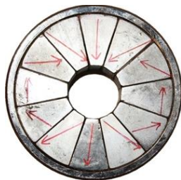
Fig. 6. Example of Halbach magnetic matrix with K=1
