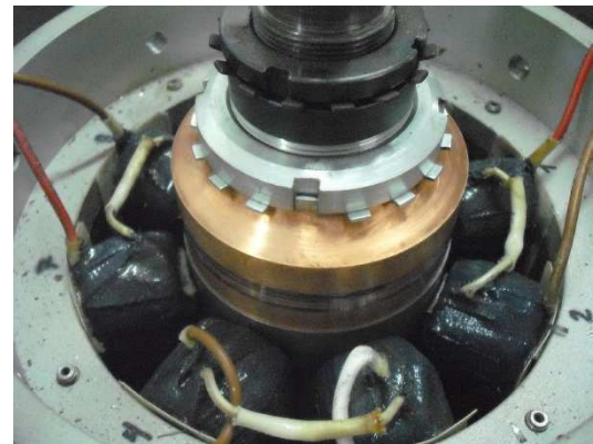
Fig. 2. Heteropolar radial active magnetic bearing
