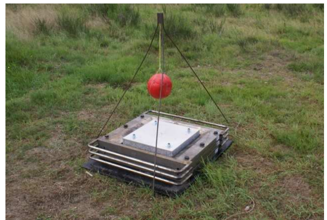
Fig. 10. The SPS system before 6 kg TNT blast test
