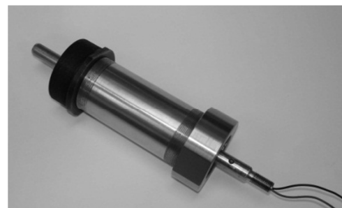
Fig. 1. View of the T-MR SiMR 132 DG damper prototype
