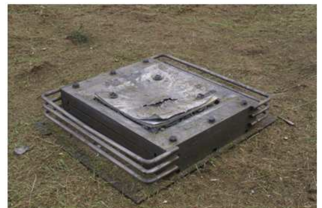
Fig. 11. The SPS system after 6 kg TNT blast test
