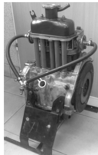
Fig. 11. The modified engine FIAT 126 650cm 3
