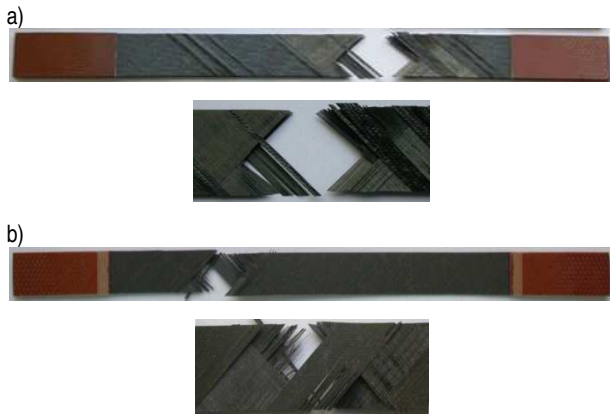
Fig. 1. Specimens of carbon/ epoxy composites after shear test: a) static test; b) fatigue test
