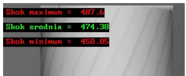
Fig. 9. Presentation of the result of rope pitch length measurements
