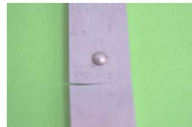
Fig. 2. Fatigue crack of the sheet with a hole riveted with mushroom rivet
