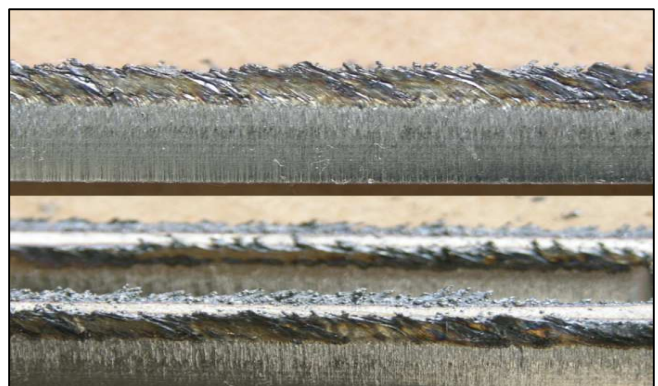
Fig. 5. Burr on cutting edges
