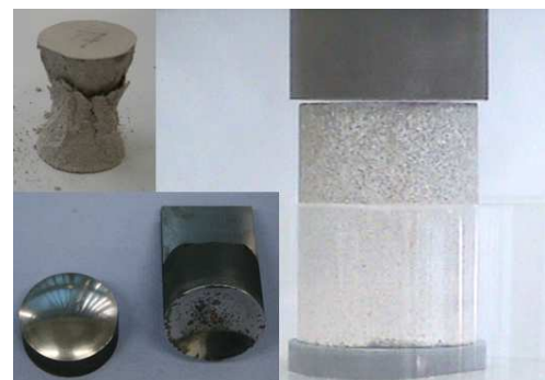
Fig. 6. The head used during the compression tests
