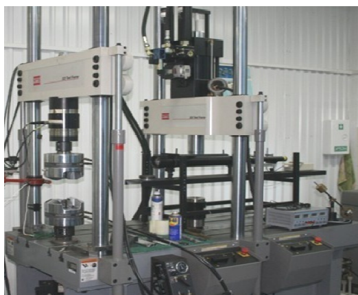
Fig. 3. The materials testing machine MTS 322
