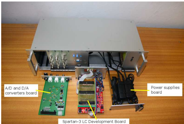
Fig. 2. Active magnetic bearings controller hardware
