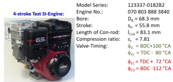
Fig. 4a. Test-engine Briggs & Stratton Intek Pro 206
