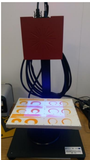
Fig. 10. Digitised sample of paint paths within the measurement area of the optical scanner
