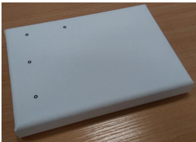
Fig. 3. Canvas ground with reference markers applied
