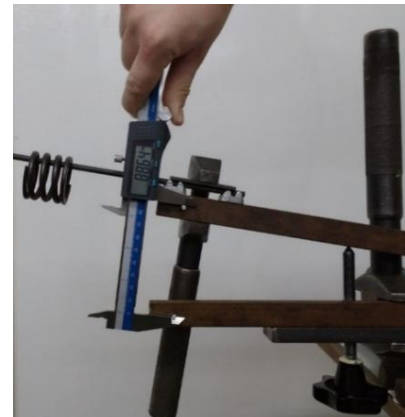
Fig. 6. Measurement of the friction coefficient for steel-steel friction pair
