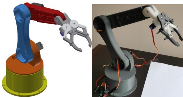
Fig. 4. Model view of the first manipulator (left side) and view of the finished construction of the first manipulator (right side)
